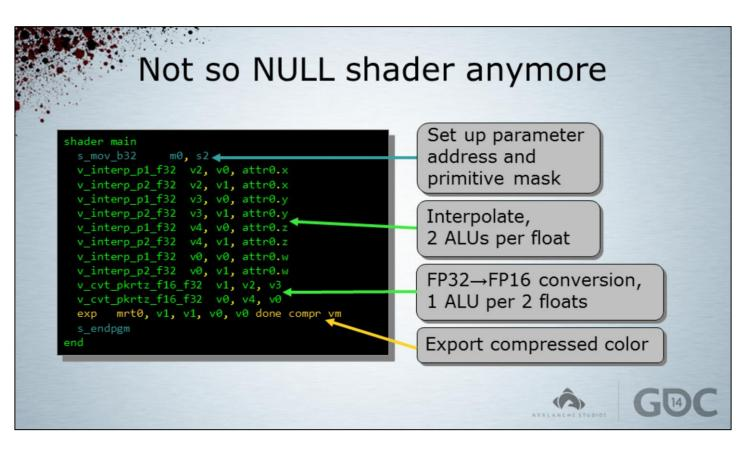
The simple pass-through shader from DX10 has now become a bunch of work to be done by the shader cores.
