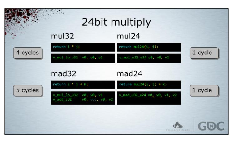
As mentioned, 24bit multiply is full rate whereas 32bit is quarter rate. The difference is further expanded when you also need to add as well. The addition can be merged into a 24bit MAD, whereas no such instruction exists for 32bit multiplies. This makes 32bit multiply-add 5 times slower than 24bit.
