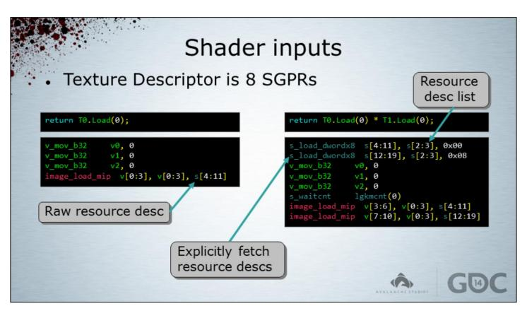
In the case of a single texture, the shader can use a raw resource descriptor. With two textures, the driver has to create a list of texture descriptors in memory and provide a pointer to it. Then the shader must load the texture descriptors from that table before it can access the textures.
