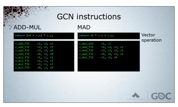
Finally, when using a vector, the extra overhead from GCN limitations can be amortized and still result in a substantial overall improvement. Instead of cutting down this float4 add-multiply from 8 to 4 operations as on previous hardware, we only go from 8 to 5, but that is still a good improvement. While we would not see a benefit on a single float in MAD-form here, even with a two-component vector would begin to see an improvement.
