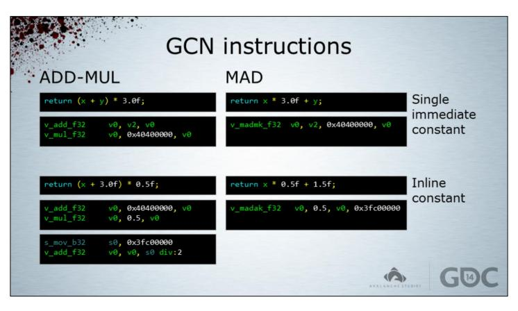
This illustrates two cases where writing in MAD-form is still beneficial on GCN. The first case only needs a single immediate constant, so this case works. Note that the left and right panels are not equivalent code, but just illustrates the difference between these forms.
