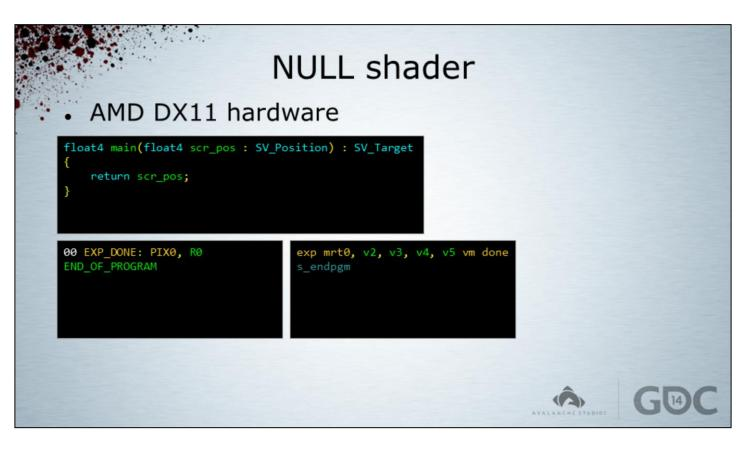
To create a NULL shader on DX11 one could simply return the screen position system value instead. These values still come preloaded in registers. On GCN we can see that they were loaded into registers v2-v5. The registers v0 and v1 usually hold the barycentric coordinates used for interpolation (not used here though).
